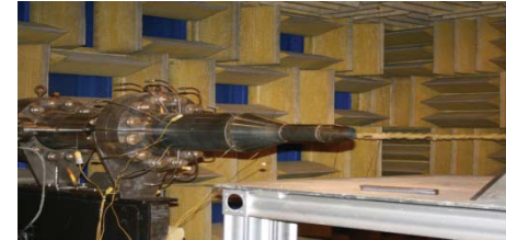
1/10 scale F414 engine, Univ. of Mississippi's National Center for Physical Acoustics
