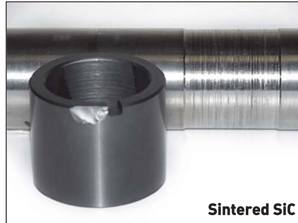
Excessive wear to a depth of 0.85 mm
